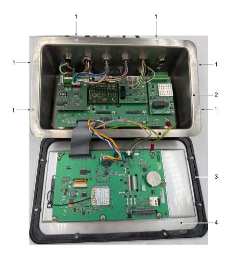
1. Loosen the 8 M4 cap nuts (1) using a 7 mm socket wrench, carefully remove the cover (4) and set aside.
