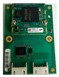
The communication interface "Anybus® CompactCom™ 40 Brick DeviceNet" (item number AB6671) from HMS is integrated into the fieldbus module. Technical data can be found on the HMS website.
