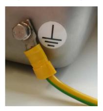
The functional ground must be connected as shown, see position G in Overview of connections.
