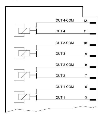
There is a jumper for each of the four relay outputs (OUT 1, OUT 2, OUT 3, OUT 4).
