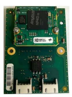
The communication interface "Anybus® CompactCom™ 40 Brick PROFIBUS" (item number AB6670) from HMS is integrated into the fieldbus module. Technical data can be found on the HMS website.
