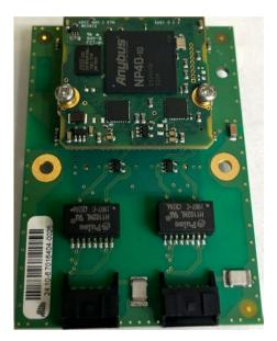
The communication interface "Anybus® CompactCom™ 40 Brick PROFINET IRT" (item number AB6675) from HMS is integrated into the fieldbus module. Technical data can be found on the HMS website.
