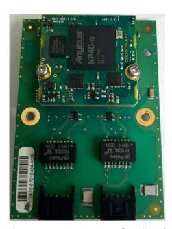
The communication interface "Anybus® CompactCom™ 40 Brick EtherNet/ IP" (item number AB6674) from HMS is integrated into the fieldbus module. Technical data can be found on the HMS website.
