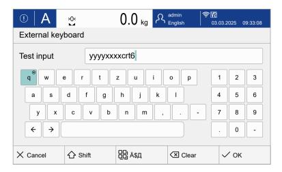
3. Use the external keyboard or barcode scanner to enter or read in any characters and check the display in the input window.
