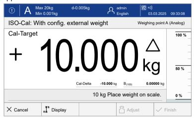
The weight display shows the calibration weight to be used (Cal target)
