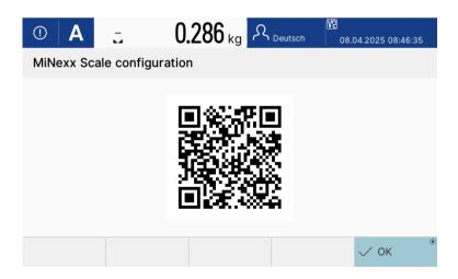
2. Scan the QR code to display and save the data on a mobile device.
